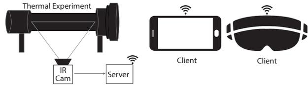
**Figure 3: The architecture of the prototype. Thermal data of an experiment is captured using an infrared camera (IR Cam) and streamed via a server to either a smartphone or HMD.**
